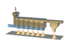
Por specialised sand, for example for foundries, power stations and mortar, an advanced process is used to make the sorted sand completely dry. It is also sorted further into special fractions at this stage and then cooled to the right temperature. The sand is now clean, dry and completely free of dust.
